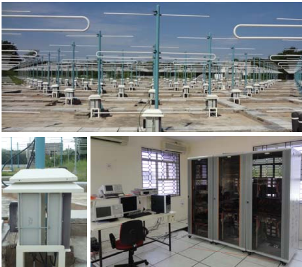
Figure-2: Photographs of the pilot active phased antenna array (top), individual TR Module (bottom left) and Control & Instrumentation (bottom right)
